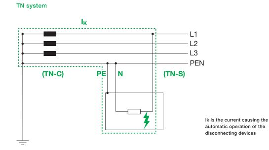
To provide a protection for TN systems with automatic disconnection of the circuit, according to IEC 60364-4 requirements, the following condition shall be fulfilled:
