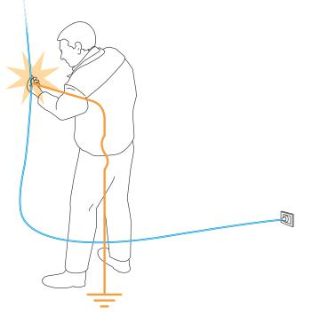
**Indirect contact:** an electric shock is received from contact with something that is connected to the electrical installation which normally is not expected to be live, but has become so as a result of a fault.
