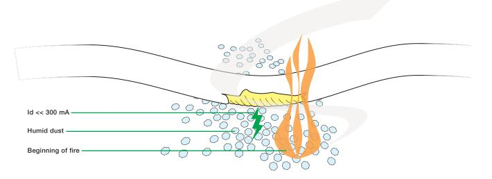
Some tests have shown that a very low leakage current (few mA) can evolve and, from 300 mA, it may set a fire in humid and dusty environments.
