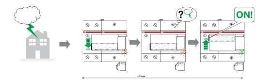
When the RCCB trips in presence of an insulation fault, the auto-reclosing device does not allow re-closing.
