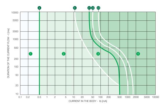
Figure 1: Time-current zones of the effects of alternating current on the human body
