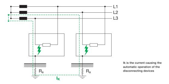
A second earth fault on an IT system (unless occuring on the same conductor as the first fault) results in a phase-phase or phase-to-neutral fault, and whether occurring on the same circuit as the first fault, or on a different circuit, overcurrent protective devices would normally operate an automatic fault clearance.
