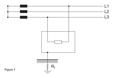
The earth fault current returns to the power supply node through the earthing arrangement of the exposed conductors and the line conductors earth capacities.
