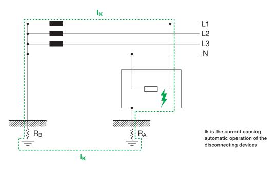
Protection by automatic disconnection of the supply used in TT system is with RCDs of sensitivity:
